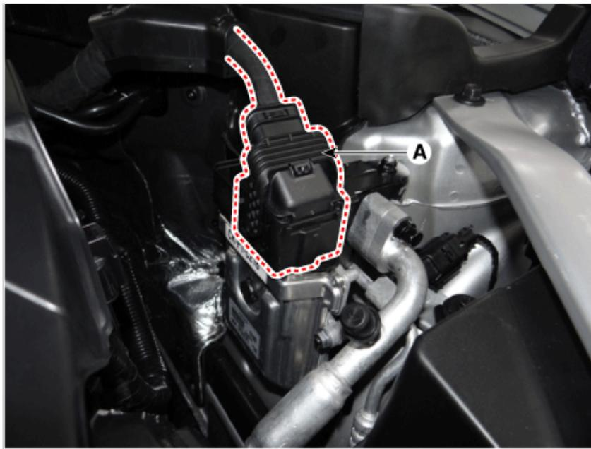
3. Remove the TCM (A) after loosening the nuts.
